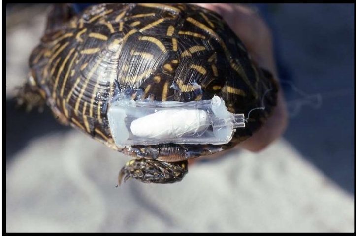
FIG. 2. An example of a bobbin thread-trailer attached to an adult Florida Box Turtle ( Terrapene carolina bauri ). This device is made of flexible plastic tubing and contains a cocoon bobbin of white thread. One end of the tubing is sealed with aquarium sealer, and the apparatus is attached to the shell with the same aquarium sealer. Photographed by C. Kenneth Dodd, Jr. and used with permission.
